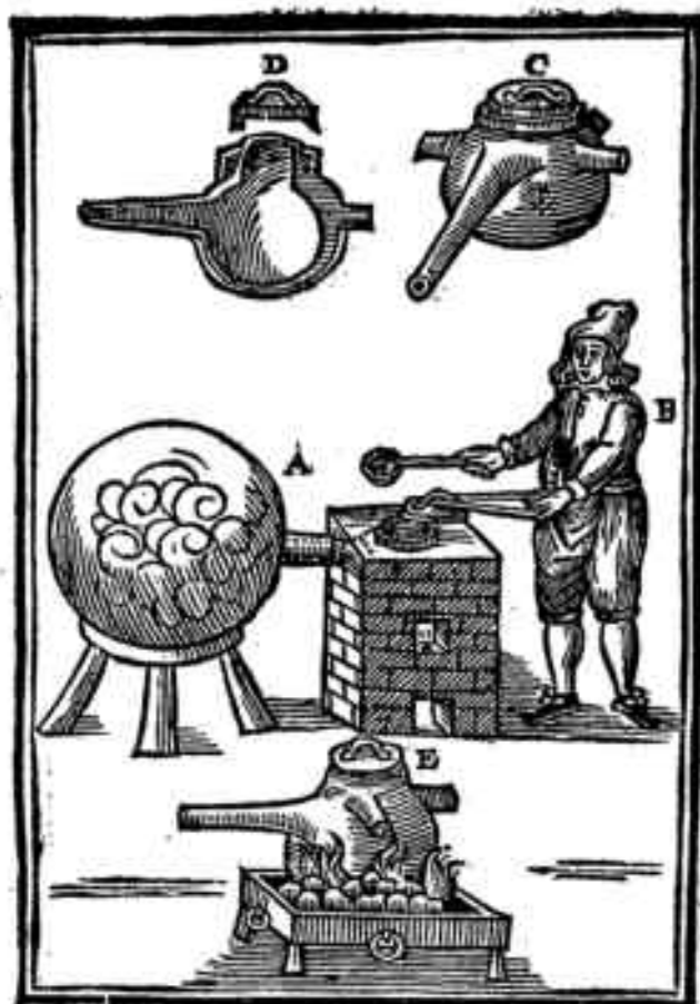
A. The furnace together with the iron distilling-veffel fastened into it, whereunto a receiver is applyed. B. The distiller with his left hand taking off the lid, and with his right casting in his prepared matter. C. The external form of the distilling vessef. D. The internal form of the vessef. E. Another distilling vessef, which is not fastened to a furnace, but only standeth upon coals.
